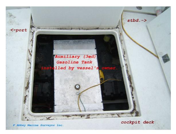
The installation of this auxiliary gasoline fuel tank at first look (through the opened deck hatch) appeared crude but possibly benign: However stepping into the hatch down into the bilge revealed significant issues, with the installation of this auxiliary gasoline tank and the later found fuel transfer system, that are not in compliance with; *The Code of Federal Regulations (33 CFR, Subpart J, Sections 183.501 - 183.590.)* as follows:
